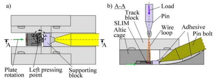
Fig. 7. Schematic representation of the cross crown fabrication tool; a) top view; b) cross section [5].
