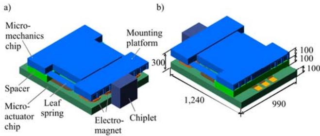
Fig. 1. Schematic representation of a Slider with an Integrated Microactuator (SLIM); a) diagonal rear view; b) diagonal front view [1].
