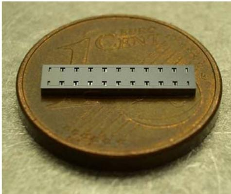
Fig. 2. Double row bar with twenty SLIM devices on a one Euro Cent coin.
