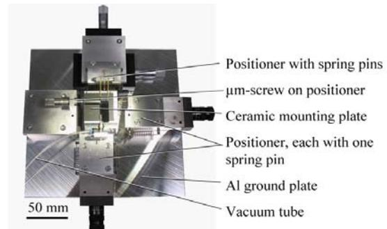
Fig. 5. Mounting set-up for chiplet bonding.
