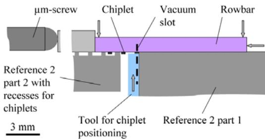
Fig. 6. Schematic detail view of mounting plate for chiplet bonding.
