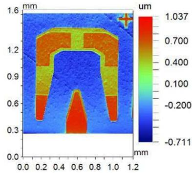
Fig. 4. Fabricated ABS-structure, measured with a white light interferometer.
