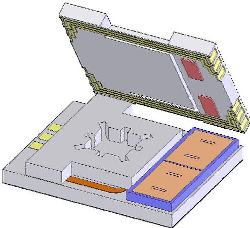
Fig. 3. Alignment and adhesive bonding of SLIM components.
